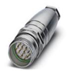
Coupler connector, with Pg11 connection thread, straight, shielded: yes, Screw locking, M23, No. of pos.: 17, type of contact: Pin, Crimp connection, cable diameter range: 3 mm ... 10.5 mm
