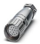
Cable connector, with Pg9 connection thread, straight, shielded: yes, Screw locking, M23, No. of pos.: 12, type of contact: Socket, Solder connection
