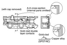
• The contact arrangement is available in two types, the SPST-NC and the SPST-NO.
