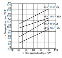
4. Ambient temperature characteristics Tested sample: AHES3191, 6 pcs.
