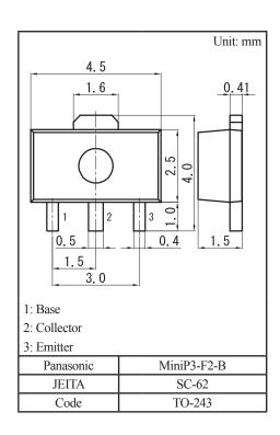
Note) \*1: Printed circuit board: Copper foil area of 1 cm<sup>2</sup> or more, and the board thickness of 1.7 mm for the collector portion Absolute maximum rating without heat sink for P<sub>C</sub> is 0.5 W
