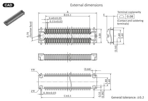
\*Because the soldering terminal Y and Z are the unified structure, they are connected electrically.
