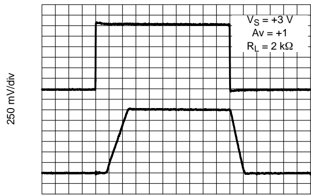
Figure 24. 3 V Non-Inverting Large Signal Pulse Response
