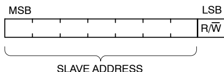
Figure 31. First Byte after START Procedure
