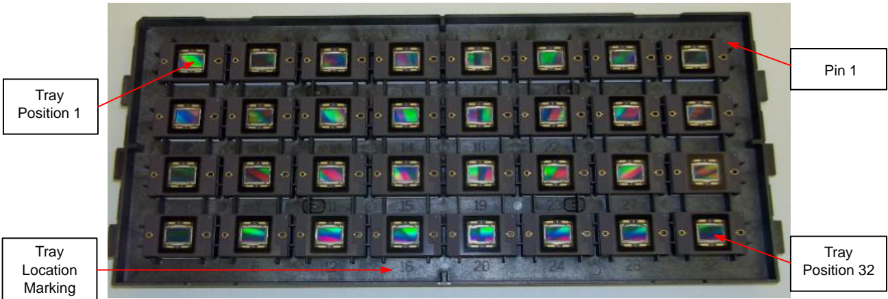
Figure 38. Tray Pin-Down View
