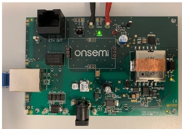
Figure 1. Operational NCP1081REF12VC4GEVB showing Basic Interconnections
