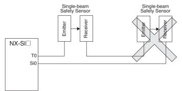
4. The total wiring length for the E3ZS Single-beam Safety Sensors is 100 m max.
