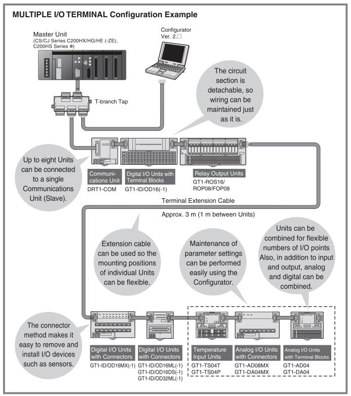
By using the DeviceNet Configurator (sold separately), control can be performed for up to 32,000 points for CJ1W-DRM21 and CS1W-DRM21-V1 DeviceNet Units, and 4,800 points for C200HX/HG/HE Master Units.
