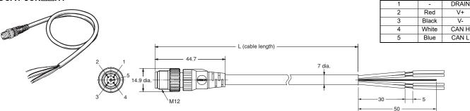
**T-branch Connector Connectors with Terminating Resistance** Wiring **DCN2-1** DRS2-1 (Plug) **Connections Diagram** Wiring Pluo CN0 (IN) Socket CN2 (OUT) Terminal No. Name DRS2-2 (Socket) Terminal No. SHIELD V+ 2 3 V-3 CAN H 4 4 12345 5 CAN L 5 Socket CN1 (OUT) Note: Terminating resistance  $(121 \Omega)$  is connected between terminals 4 and 5. (56) 4.5 dia. •13.6• 17.7 -24.7 8 dia. (Countersinking: 2) **+**-12-44.7 10 OT CNO 13.6
