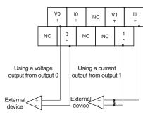
**Note:** The voltage and current output ranges (signals) are set with either the DIP switch or the Configurator settings.
