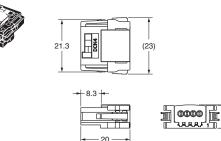
Power Supply Terminal Block with Terminating Resistance for Flat Cable DCN4-TP4D
