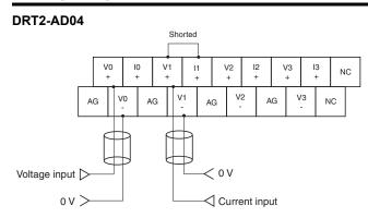
Note: With using a current input, always short the V+ and I+ terminals. (Use the shorting bar provided with the Unit.)
