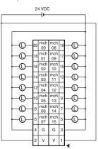
MIL Connector Terminals with Transistors DRT2-D32ML(-1)/D16ML(-1)
