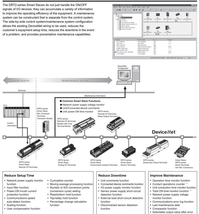
\* The number of contact operations monitor function and the cumulative ON time monitor function cannot be used simultaneously for the same contact.
