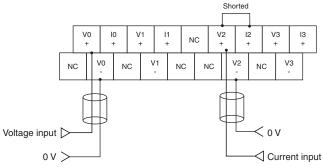
Note: With using a current input, always short the V+ and I+ terminals. (Use the shorting bar provided with the Unit.)
