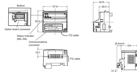
After the DeviceNet Communication Unit is installed dimension D of the inverter increases by 26.4 mm (Dimension D of the inverter varies depending on the capacity. Refer to the MX2-series USER'S MANUAL (Cat.No.I585))
