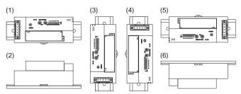
A current of 0.35 mA flows to sensors connected to the DRT2-TS04P. The indicator accuracy specifications differ depending on the mounting direction. Refer to the above table for details.
