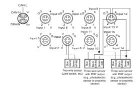
**Environment-resistive Terminals with Transistors (Standard Type)**
