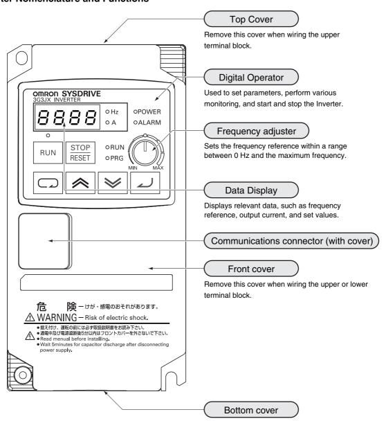
Remove this cover when wiring the lower terminal blocks.
