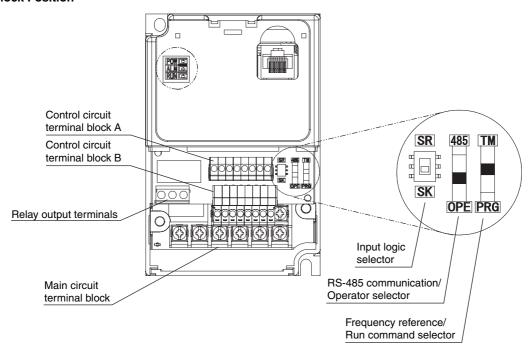
Note. This illustration shows the terminal block with the front cover removed
