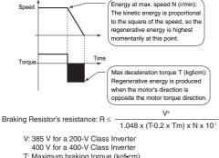
T: Maximum braking torque (kgf•cm) Tm: Motor's rated torque (N•cm) N: Maximum speed (r/min)
