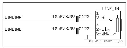
The socket can interface standard 3.5 mm phone connector (also known stereo plug or audio plug).
