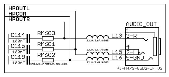
The connector can interface standard 3.5 mm phone connector (also known stereo plug or audio plug).
