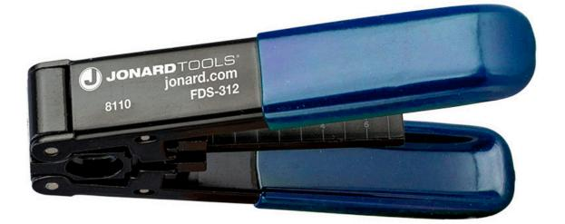
Specifically designed to strip 3.1mm(W)x2.0mm(H) FTTH drop cables, this tool strips the outer jacket of drop cables and cuts the strength members exposing the fiber inside. This drop cable stripper features the following:
