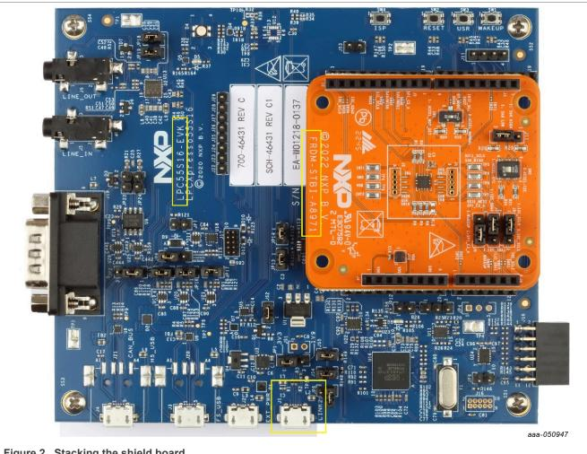
Figure 2. Stacking the shield board
