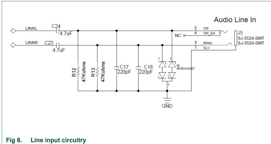
Fig 6. Line input circuitry
