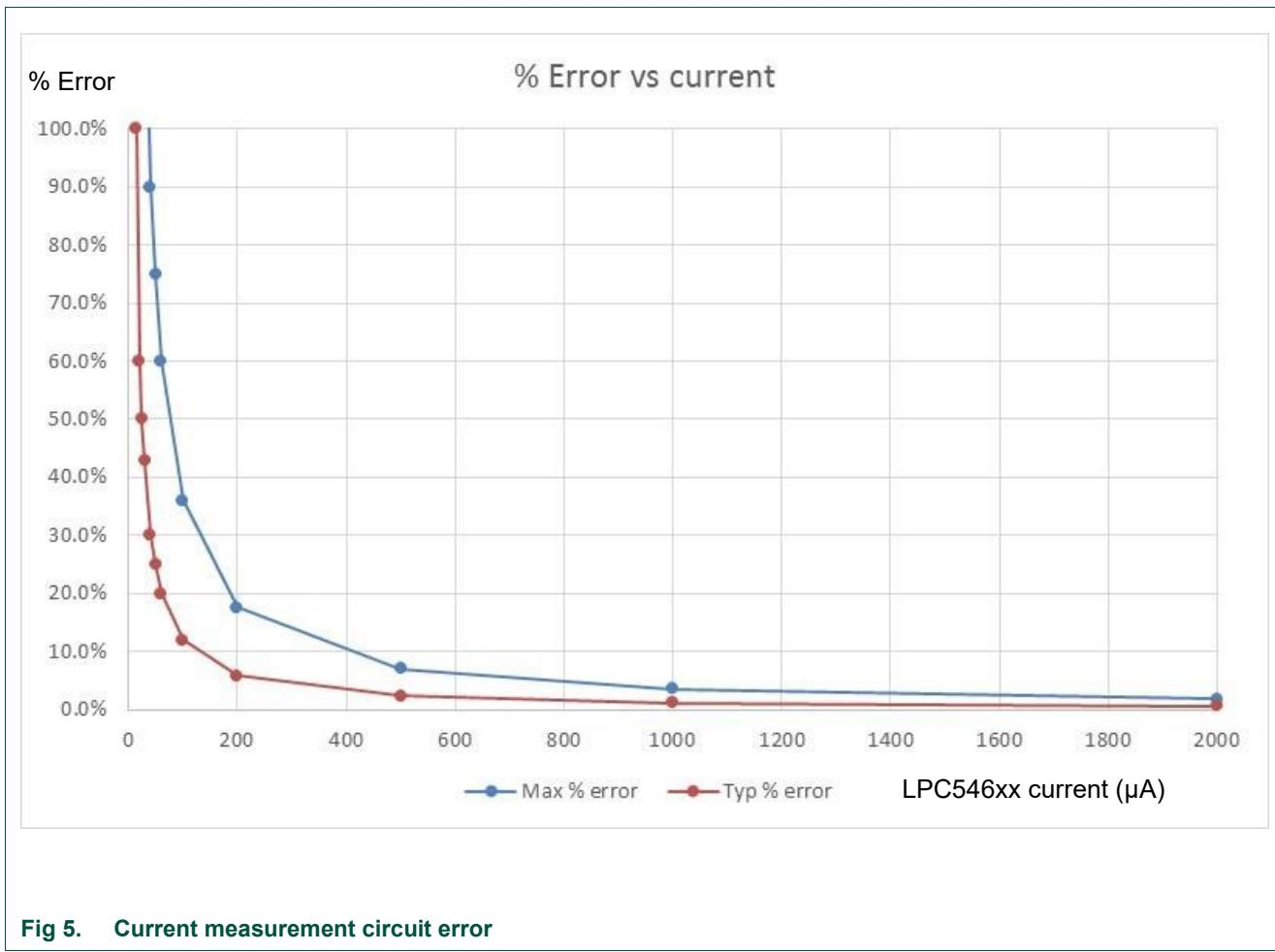
**Fig 5. Current measurement circuit error**
