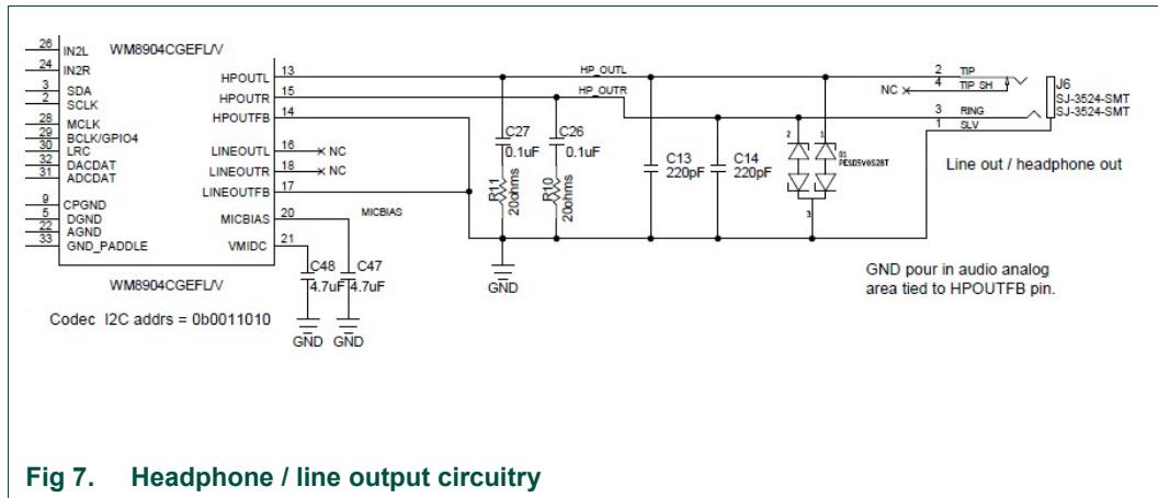
Fig 7. Headphone / line output circuitry
