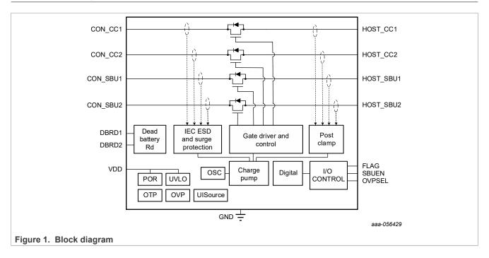
48 V Type-C CC and SBU protection IC for USB PD EPR
