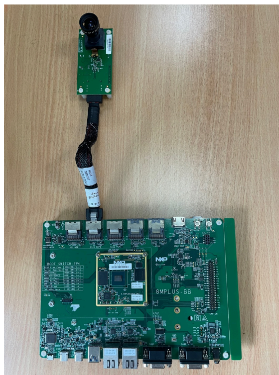
Figure 2. Hardware setup of IMX-OS08A20 accessory card
