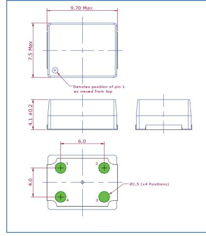
Recommended Land Pattern  $\begin{array}{r} 6.0 \\ \hline 01.5 (x4) \\ \hline 0 \\ \hline 0 \\ \hline \end{array}$   $\begin{array}{r} \hline 1 \\ \hline 1 \\ \hline 0 \\ \hline 2 \\ \hline \hline 0 \\ \hline \end{array}$ Note: For correct operation, decouple the supply voltage with a 10 µF capacitor close
