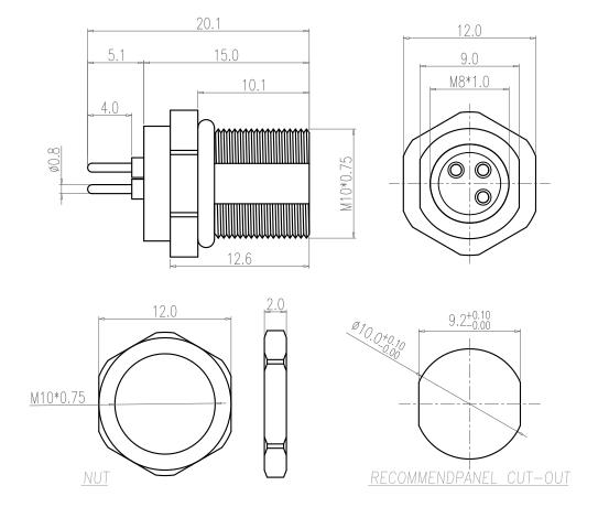
NOTE: MATERIAL HOUSING: PA66 UL94V-0, BLACK CONTACT: BRASS NUT: BRASS SHELL: **BRASS DRING**: **EPDM** FINISH CONTACT: 10u" GOLD PLATED OVER NICKEL NUT: NICKEL PLATED SHELL: NICKEL PLATED **ELECTRICAL** RATED CURRENT: ЗА 60V RATED VOLTAGE: INSULATION RESISTANCE: 100 MOhms MIN. CONTACT RESISTANCE: 10 mOhms MAX. WATER PROOF: IP67 **ENVIRONMENT OPERATION TEMPERATURE:** -40°C TD +85°C
