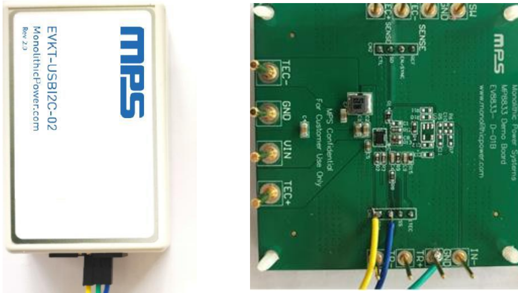
Figure 6: EVB to MPS I 2 C Communication Interface Wire Connection
