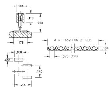
Interconnect Socket Surface Mount Socket Accepts .015"- .025" (0,38 - 0,635 mm) dia leads Single Row Surface Mount **Plating Code:** 41 Shell Plating: 200 µ" Tin (matte finish) over 100 µ" Nickel Inner Contact Plating: 10 µ" Gold over 50 µ" Nickel
