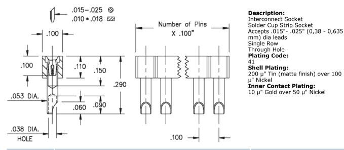
Mill-Max **RoHS** Of Compliant Part **Pins** Number
