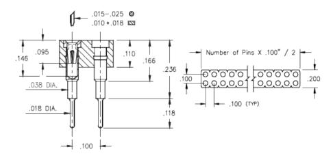
**Description:** Interconnect Socket Elevated Strip Socket Accepts .015"- .025" (0,38 - 0,635 mm) dia leads Double Row Through Hole Plating Code: Shell Plating: 200 µ" Tin (matte finish) over 100 μ" Nickel
