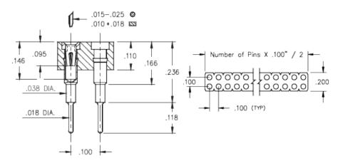
**Description:** Interconnect Socket Elevated Strip Socket Accepts .015"- .025" (0,38 - 0,635 mm) dia leads Double Row Through Hole Plating Code: Shell Plating: 200 μ" Tin/Lead(93/7) over 100 μ" Nickel
