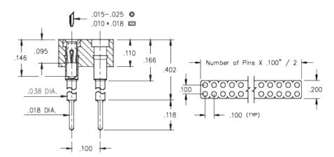
**Description:** Interconnect Socket Elevated Strip Socket Accepts .015"- .025" (0,38 - 0,635 mm) dia leads Double Row Through Hole Plating Code: **Shell Plating:** 200 μ" Tin/Lead(93/7) over 100 μ" Nickel Inner Contact Plating:
