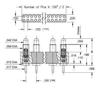
**Description:** Interconnect SLC Header Spring-Loaded Header Vertical Mount Through-Hole Double Row Through Hole Plating Code: Shell Plating: 20μ" Gold over 100μ" Nickel Inner Spring Plating:
