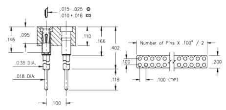
**Description:** Interconnect Socket Elevated Strip Socket Accepts .015"- .025" (0,38 - 0,635 mm) dia leads Double Row Through Hole Plating Code: Shell Plating: 200 µ" Tin (matte finish) over 100 μ" Nickel Inner Contact Plating:
