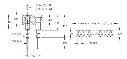
**Description:** Interconnect Socket Elevated Strip Socket Accepts .015"- .025" (0,38 - 0,635 mm) dia leads Double Row Through Hole Plating Code: Shell Plating: 200 µ" Tin (matte finish) over 100
