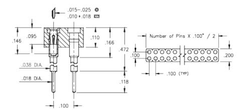
**Description:** Interconnect Socket Elevated Strip Socket Accepts .015"- .025" (0,38 - 0,635 mm) dia leads Double Row Through Hole Plating Code: **Shell Plating:** 200 µ" Tin (matte finish) over 100 μ" Nickel Inner Contact Plating:
