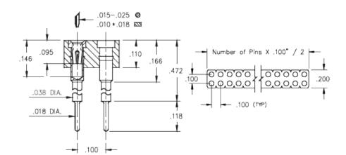
**Description:** Interconnect Socket Elevated Strip Socket Accepts .015"- .025" (0,38 - 0,635 mm) dia leads Double Row Through Hole Plating Code: Shell Plating: 200 μ" Tin/Lead(93/7) over 100 μ" Nickel Inner Contact Plating:
