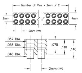
**Description:** Interconnect Target Connector Spring-Loaded Header Vertical Mount SMT Target Double Row Surface Mount **Plating Code:** 10 Shell Plating: 10 µ" Gold over 100 µ" Nickel Packaging: Packaged in Bulk
