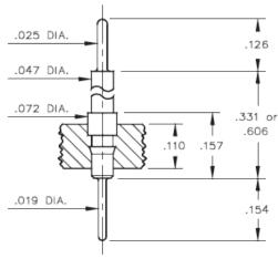
**Description:** PGA Header Solder Tail PGA Header Through Hole Plating Code: Shell Plating: 200 μ" Tin/Lead(93/7) over 100 µ" Nickel
