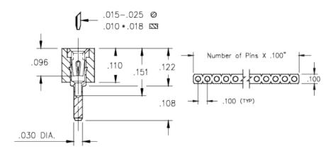
**Description:** Interconnect Socket Low Profile Solder Tail Socket Accepts .015" - .025" (0,38 - 0,635 mm) dia leads Single Row Through Hole
