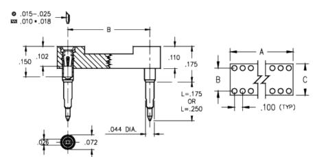
**Description:** DIP Dual In Line Socket Solderless Press-Fit Standard Tail Open Frame Through Hole Plating Code: Shell Plating: 10 μ" Gold over 100 μ" Nickel Inner Contact Plating: 10 μ" Gold over 50 μ" Nickel
