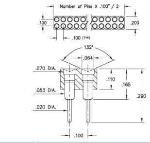
**Description:** Interconnect Concave Face Target Connector Spring-Loaded Header Vertical Mount Through Hole Target with Concave Face Double Row Through Hole Plating Code: 10 Shell Plating: 10 µ" Gold over 100 µ" Nickel Packaging: Packaged in Bulk
