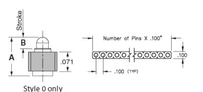
**Description:** Interconnect SLC Header Spring-Loaded Header Vertical Mount SMT Single Row Surface Mount Plating Code: 22 Shell Plating: 20µ" Gold over 100µ" Nickel Inner Spring Plating: 10µ" Gold Packaging: Packaged in Bulk
