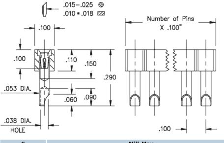
**Description:** Interconnect Socket Solder Cup Strip Socket Accepts .015"- .025" (0,38 - 0,635 mm) dia leads Single Row Through Hole Plating Code:
