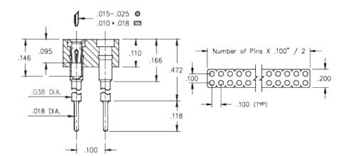
**Description:** Interconnect Socket Elevated Strip Socket Accepts .015"- .025" (0,38 - 0,635 mm) dia leads Double Row Through Hole Plating Code: **Shell Plating:** 200 µ" Tin (matte finish) over 100 μ" Nickel Inner Contact Plating: 10 μ" Gold over 50 μ" Nickel
