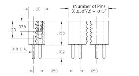
Interconnect Socket Standard Solder Tail Socket Accepts .015"- .020" (0,38 - 0,508 mm) dia leads Double Row Through Hole Plating Code: 41 Shell Plating: 200 µ" Tin (matte finish) over 100 µ" Nickel Inner Contact Plating: 10 µ" Gold over 50 µ" Nickel
