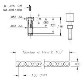
Description: Interconnect Carrier Plastic Carrier with Low Profile Receptacles Single Row Through Hole Plating Code: 43 Shell Plating: 200 µ" Tin (matte finish) over 100 µ" Nickel Inner Contact Plating: 30  $\mu^{\prime\prime}$  Gold over 50  $\mu^{\prime\prime}$  Nickel
