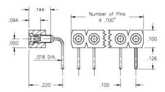
**Description:** Interconnect Socket Right Angle Socket Accepts .015" - .025" (0,38 - 0,635 mm) dia leads Single Row Through Hole Plating Code: Shell Plating: 10  $\mu$ " Gold over 100  $\mu$ " Nickel Inner Contact Plating: 10  $\mu$ " Gold over 50  $\mu$ " Nickel
