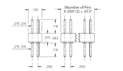
**Description:** Interconnect Header Solder Tail Pin Header .016" (0,41mm) Pin Head Double Row Through Hole Plating Code: 10 Shell Plating: 10  $\mu$ " Gold over 100  $\mu$ " Nickel
