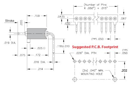
**Description:** Interconnect SLC Header Spring-Loaded Header Horizontal Mount Single Row Through Hole Plating Code:
