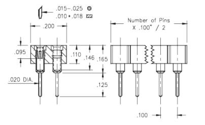
**Description:** Interconnect Socket Standard Solder Tail Socket Accepts .015"- .025" (0,38 - 0,635 mm) dia leads Double Row Through Hole Plating Code: 43 Shell Plating:
