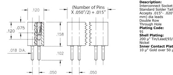
Standard Solder Tail Socket Accepts .015"- .020" (0,38 - 0,508 mm) dia leads Double Row Through Hole Plating Code: Shell Plating: 200 μ" Tin/Lead(93/7) over 100 μ" Inner Contact Plating:
