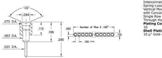
Description: Interconnect Target Connector Spring-Loaded Header Vertical Mount Through Hole Target with Concave Face Single Row Through Hole Plating Code: 10 Shell Plating:
