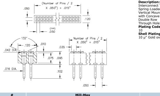
Interconnect Target Connector Spring-Loaded Header Vertical Mount Through Hole Target with Concave Face Double Row Through Hole Plating Code: Shell Plating:
